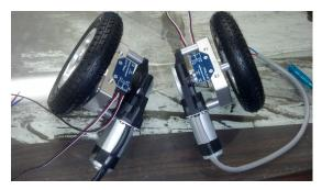
Fig. 5: Motors with 144 tick encoders
